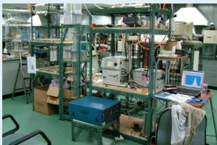
Circulating fluidized-bed system for nitrogen oxides control
