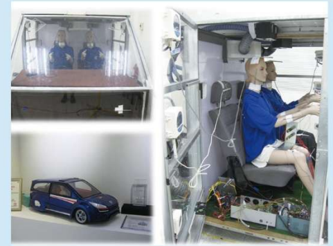
Specialized air conditioning system being tested with thermal mannequins to simulate body heat.
