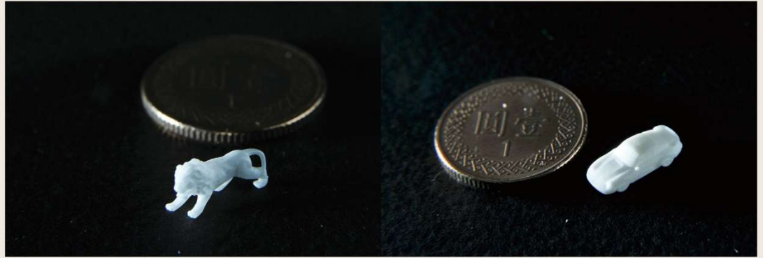
Actual finished products printed from the 3D printer. On left, miniature lion figure (approx. 1.2 x 0.3 x 0.6 cm)
