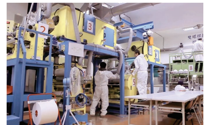
A multi-purpose coating machine designed by researchers of the Smart Textile Technology Research Center.
